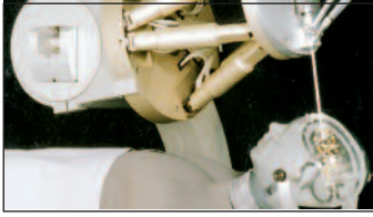
Custom Hexapod designed for neurosurgery Photo: IPA
