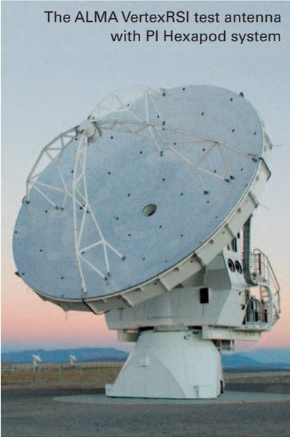
telescope. The spread of the antenna array will be between 150 m and a maximum of 12 km. On completion in 2011, ALMA will be the largest and most powerful radio telescope in the world, with a resolution ten times better than that of the Hubble space telescope.
