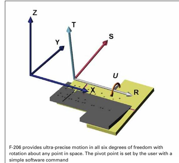
F-206 provides ultra-precise motion in all six degrees of freedom with rotation about any point in space. The pivot point is set by the user with a simple software command
